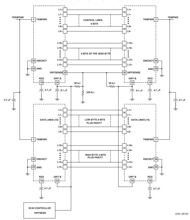
NOTE: A 220-kΩ resistor is added to ground to insure the transceivers will come up in single-ended mode when no terminator is enabled. The controller DIFFSENS ties to the DIFFB pin on the terminators, only one RC network should be on a device.
